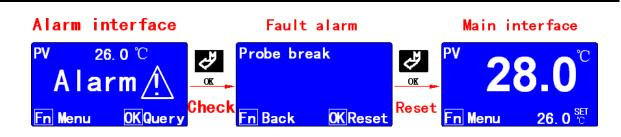
Note: After checking the fault, pls remove it first, then reset the chiller.
