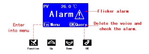
• Fault checking and Reset
